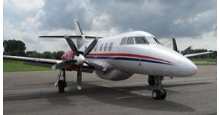
BAE System Jetstream 3100 & 3200 with 5-blade MTV-27
